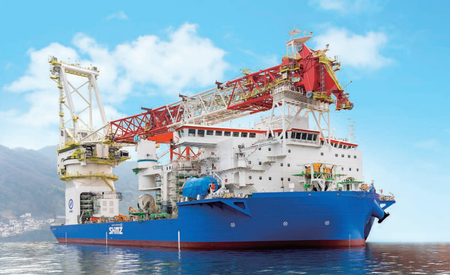
SEP* vessel for construction of offshore wind power plant (under construction) * Self-Elevating Platform
