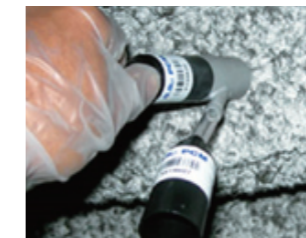
Asbestos deterioration diagnostics
