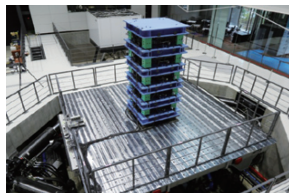
An experiment using the E-Beetle large-scale shaking table (The E-Spider large-stroke shaking table is visible in the background.)
