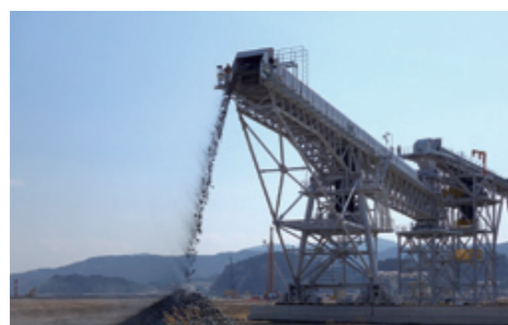
Large-scale conveyor belt used to transport earth
